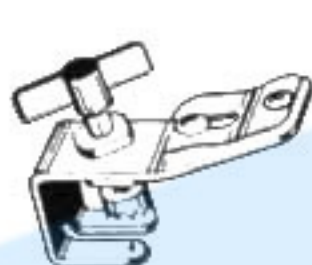
Riechert TC12-059 Fixation base, for skull mounting, holding 1 flexible arms
