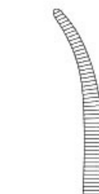
TC6-460 16cm TC6-461 20cm Narrow Jaws, longitudinal Serrations, with 1x2teeth curved
